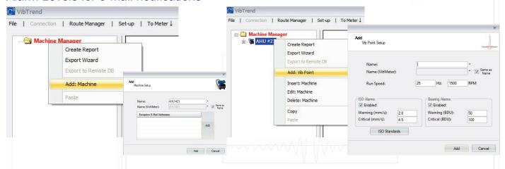
Create routes for operatives to follow and send these "To" and "From" the Meter to easily identify the measuring point and record the Vibration & Bearing Condition of the Machine
