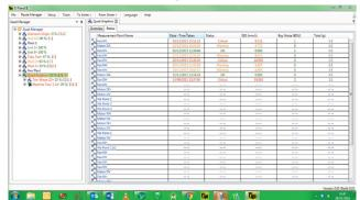
Perform further diagnosis of Machine Measuring points using a wide variety of additional features such as Crest Factor, DEMOD, Waterfall FFT, VA Bands etc...
